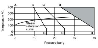
The product must not be used in this region or beyond the parameter of the PMA or TMA of the relative end connection.
